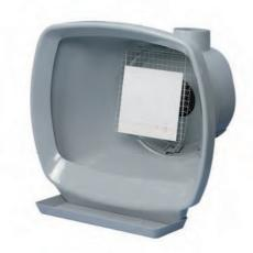
The spray box serves as protective device when spraying TLC/HPTLC plates with aggressive solutions.
